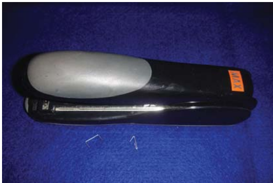
Figure 16.23 Stapler with bent and unbent staples.
